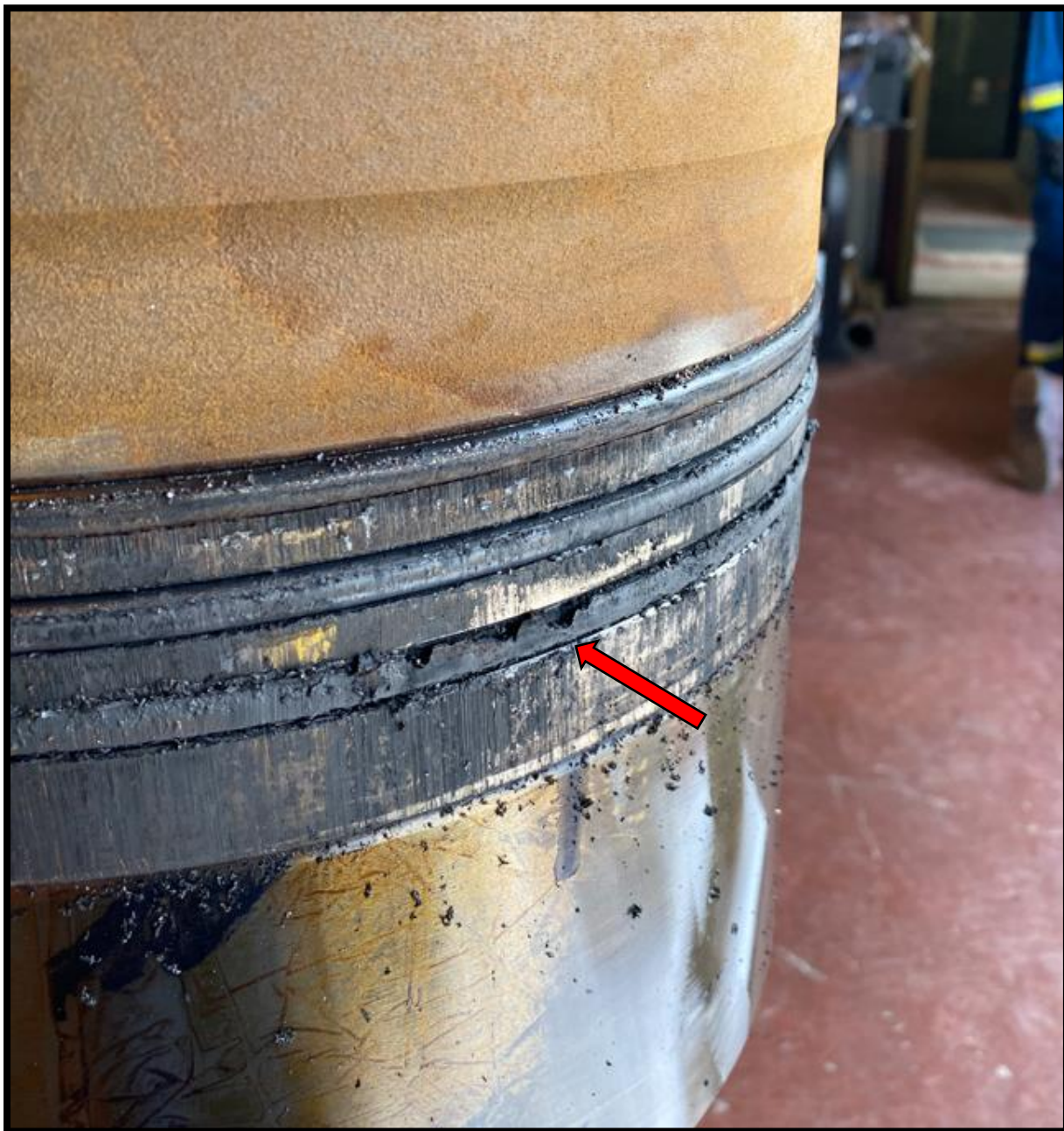
Figure 12- #4 Right Liner O-rings
