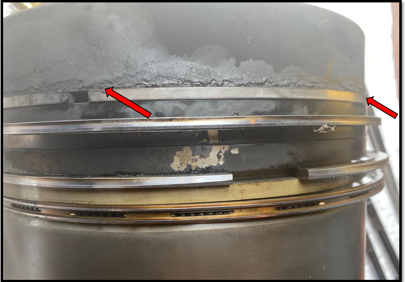
Figure 24 - Piston #5 Left - Top ring seized and flaking
