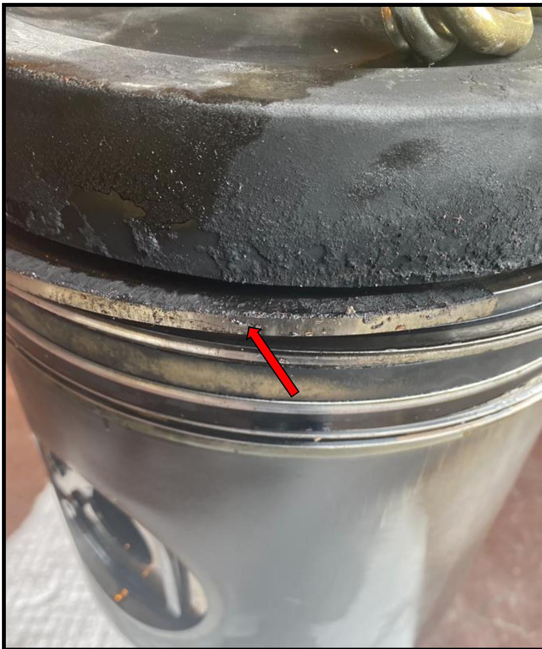
Figure 7 - #4 Right Piston - Ring with carbon
