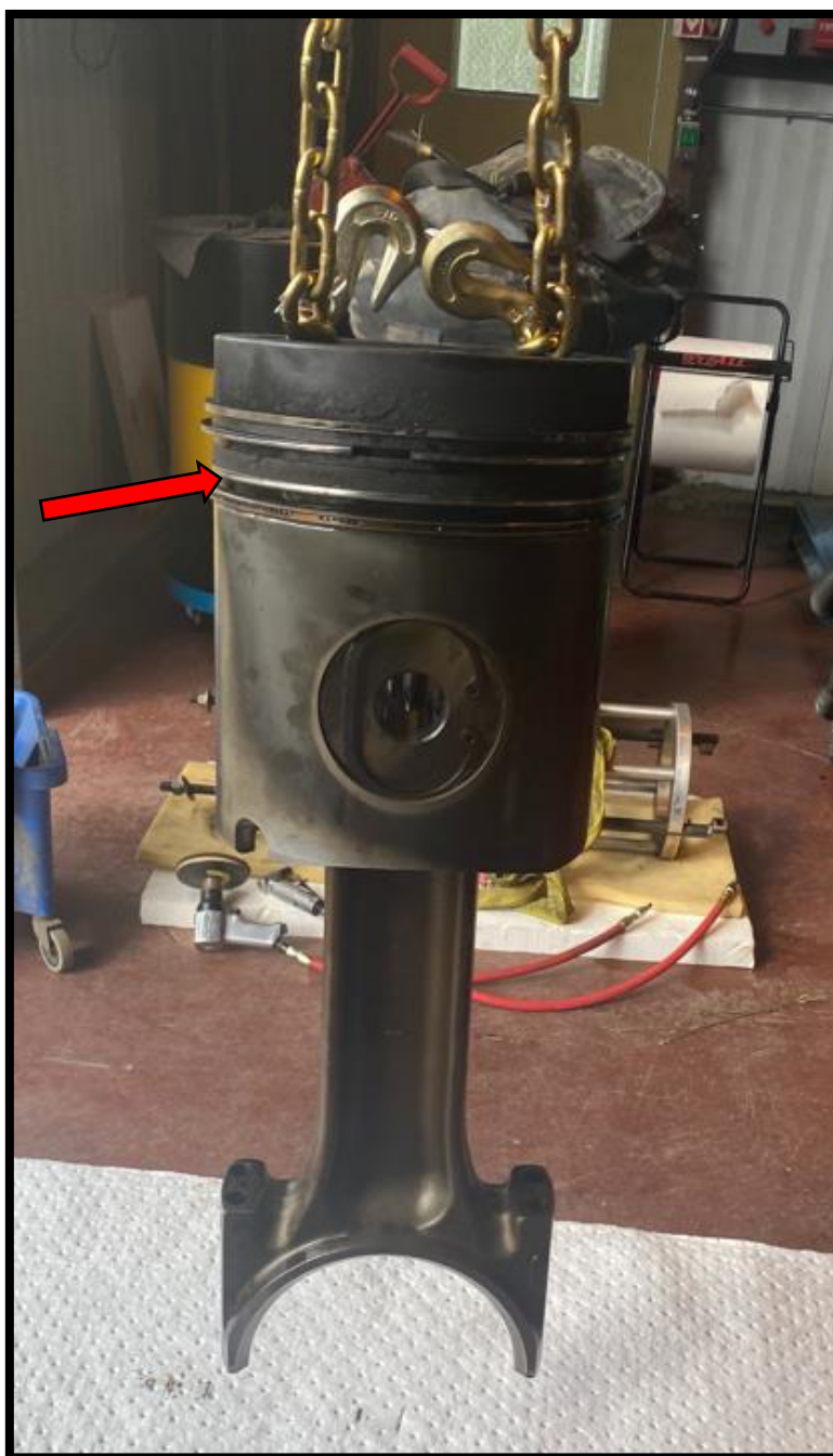
Figure 6- #4 Right Piston - Seized Third Ring
