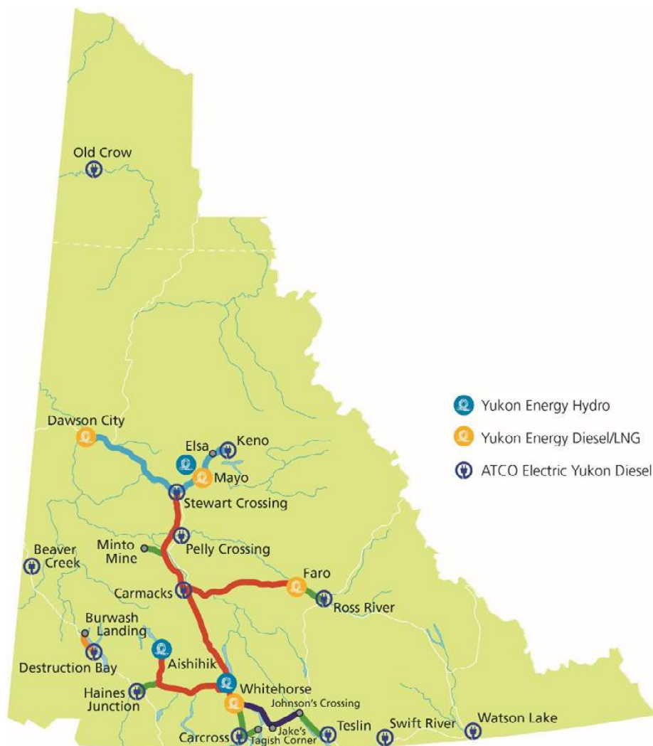
Figure 1: Yukon Electrical Systems
