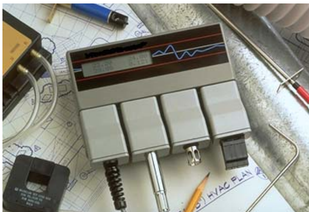
Figure 7.20: Multi-Channel Portable Datalogger
