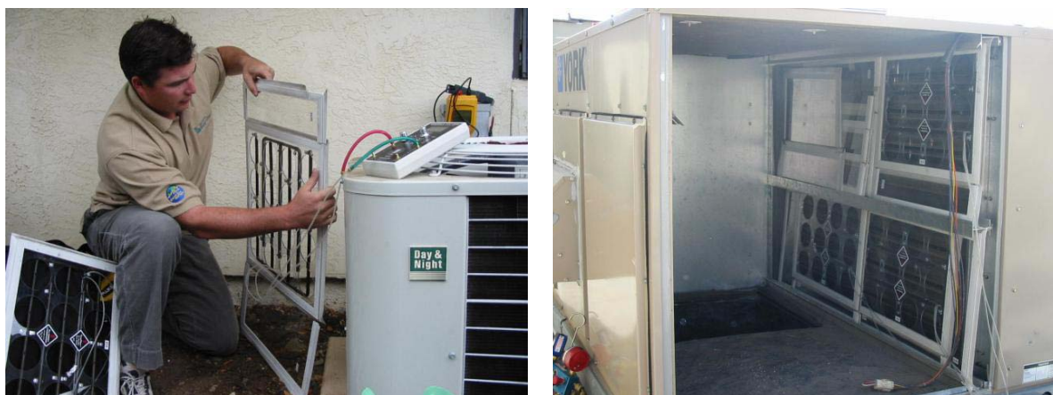
Figure 7.10: Airflow Measurements Using a Flow Grid
