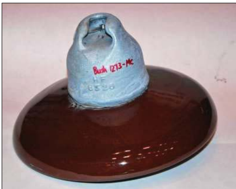
Figure 5: Example of insulator containing a small amount white crystalline deposit on cap of
