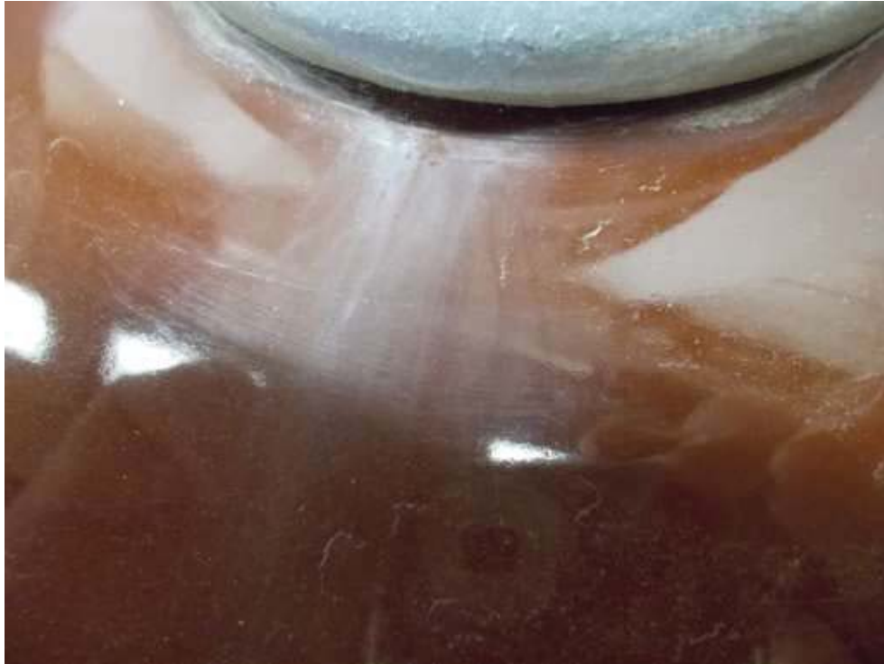
Figure 2 - Electrical activity etched in the stain,
