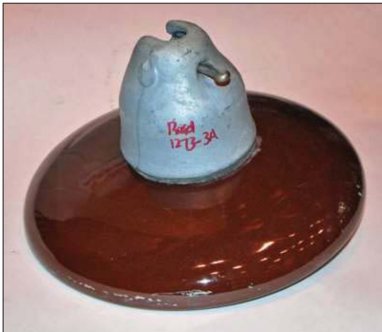
Figure 4: Overall Condition of In-Service Insulators. No apparent corrosion attack of the galvanized coating is noted in the majority of samples.
