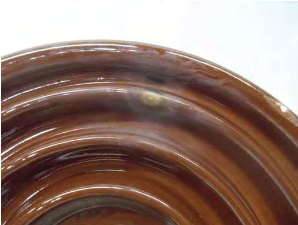
Figure 2 - Electrical activity etched in the stain,
