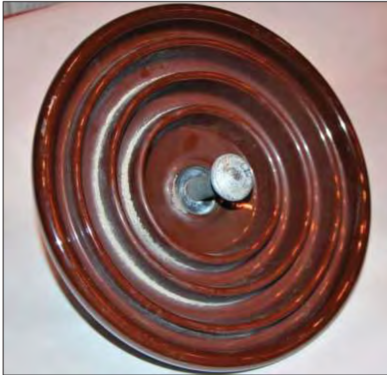
Figure 6: Debris present on underside of insulator sheds. Also note good condition of grout
