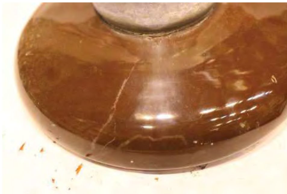
Figure 1 – Stain from the cap that extends and fades towards the porcelain edge.
