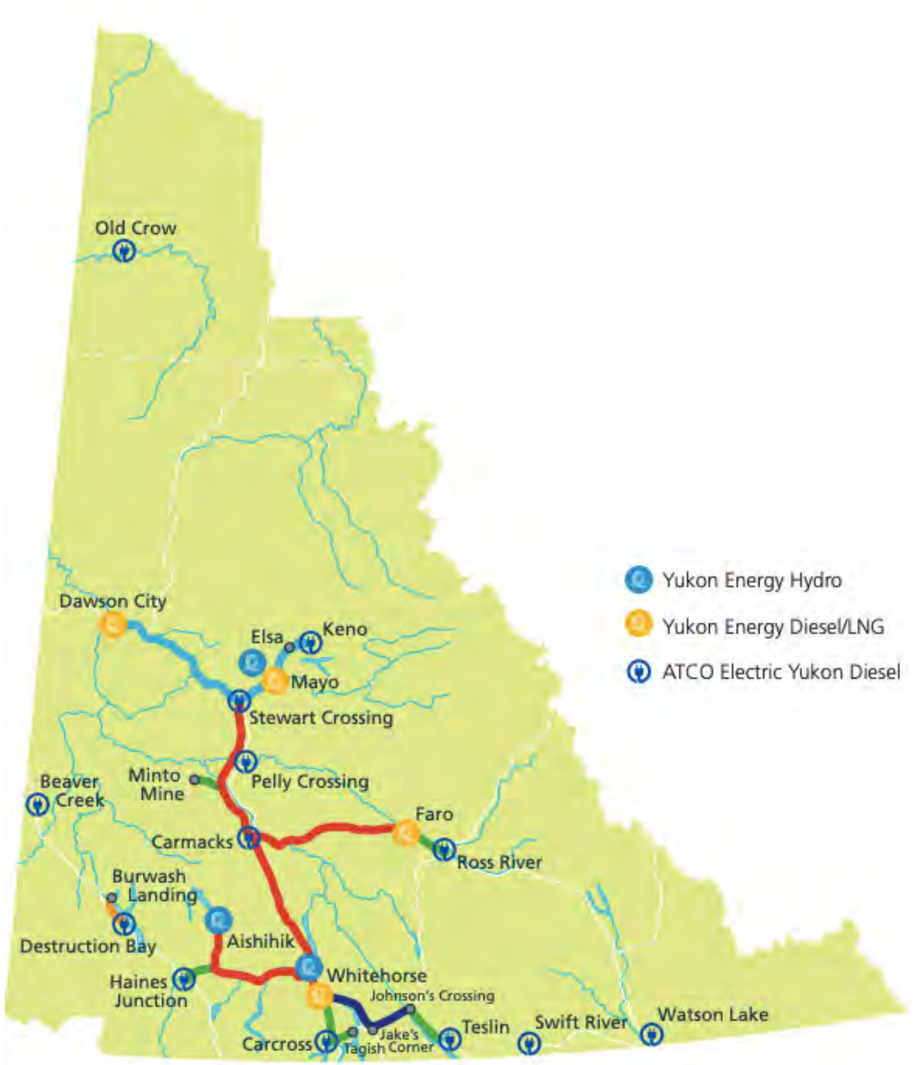
Figure 5. Yukon's electrical generation facilities and transmission lines. Figure provided by the Yukon Energy Corporation.
