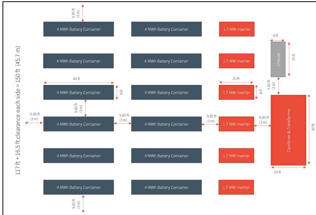
Figure 10-1: Preliminary layout for a 10 MW/40 MWh containerized BESS with 20% overbuild (total capacity 10 MW/48 MWh).
