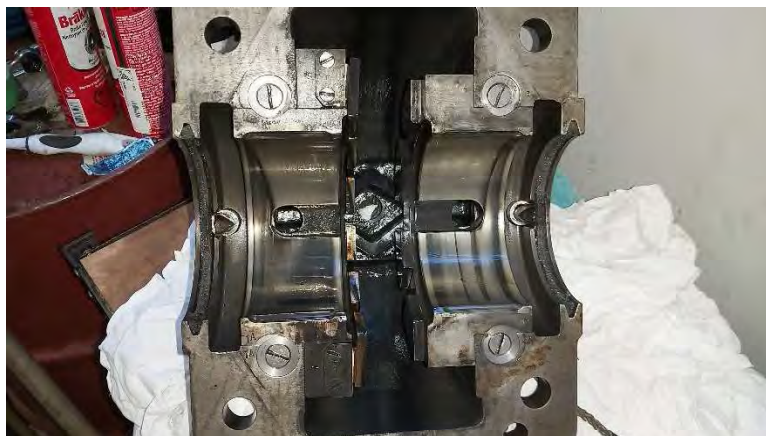
Figure 6: Turbine Journal Bearing Minor Wear
