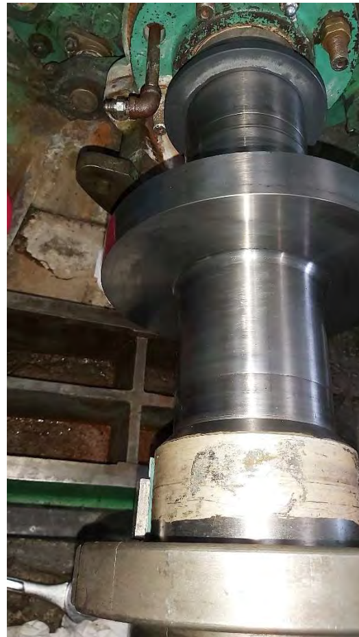
Figure 5: Turbine Journal Bearing Shaft Scoring
