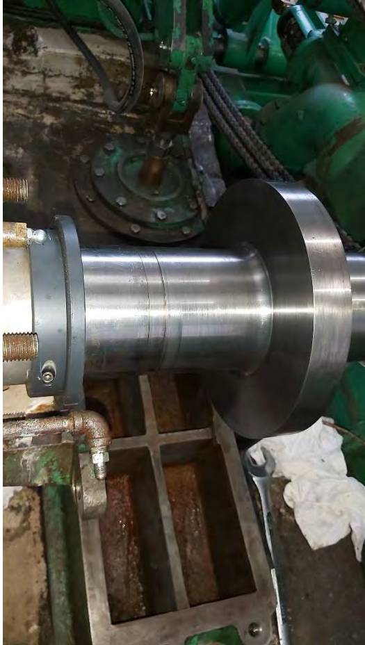
Figure 5: Turbine Journal Bearing Shaft Scoring
